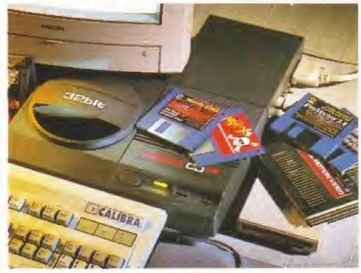
The SX-1 can cause compatibility with certain CD 32 titles if you add SIMM memory chips to your machine.
